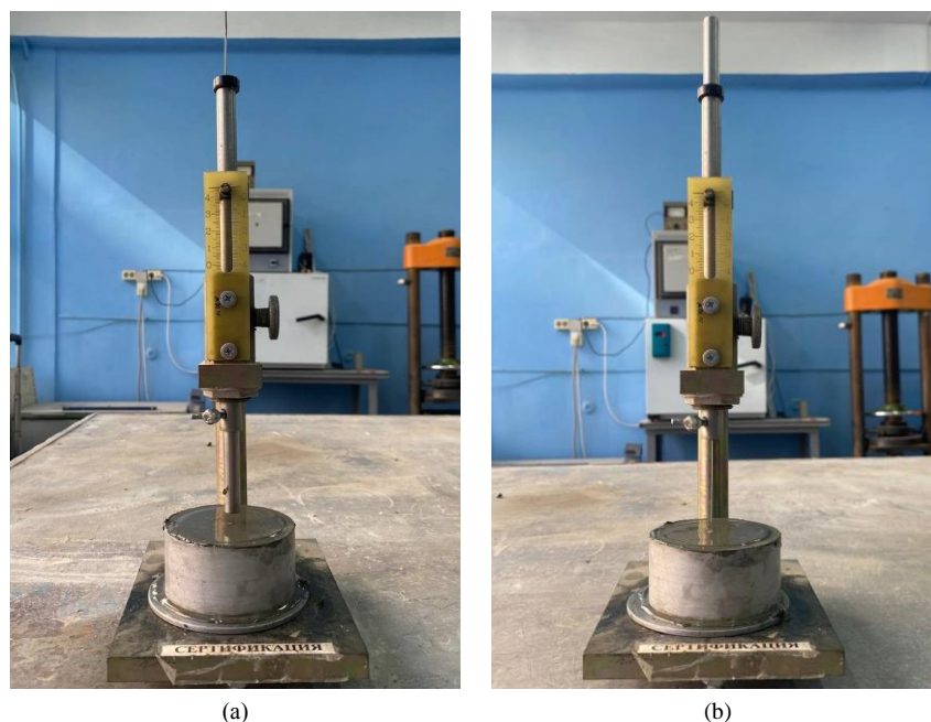
Figure 6. Testing of cement mixture samples with RSP: (a) normal consistency; (b) setting time
