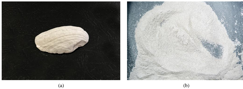
Figure 2. Appearance of RSP: (a) after washing; (b) after grinding when added to combination of concrete
