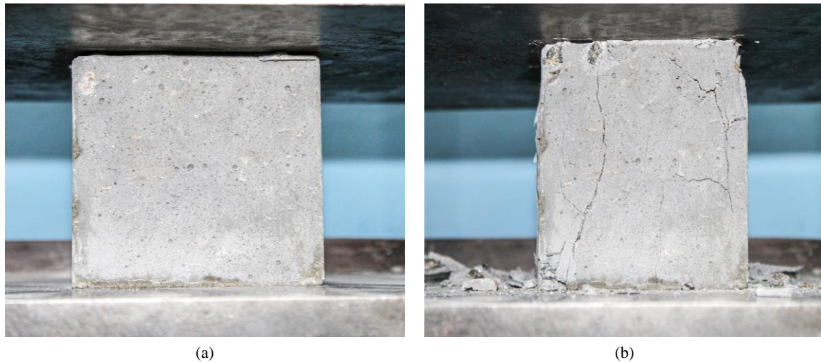
Figure 8. Determination of the R_c of samples with RSP: (a) before failure; (b) after destruction
