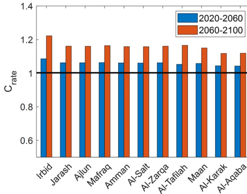
**Figure 12. Comparison of the average corrosion rate projected using RCP 8.5 forcing scenarios with the historical data along the main cities in Jordan for 2020-2060 and 2060-2100**
