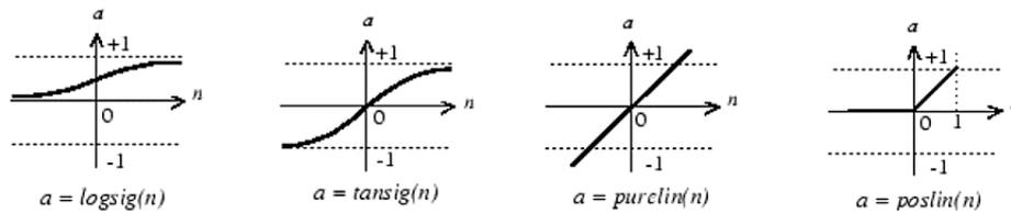
Figure 4. Various activation functions used in ANN
