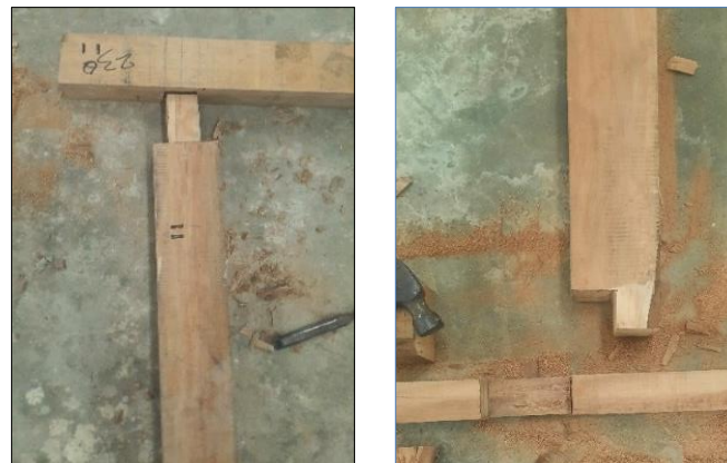
Figure 6. (a) Mortise and tenon joint. (b) Halved joint
