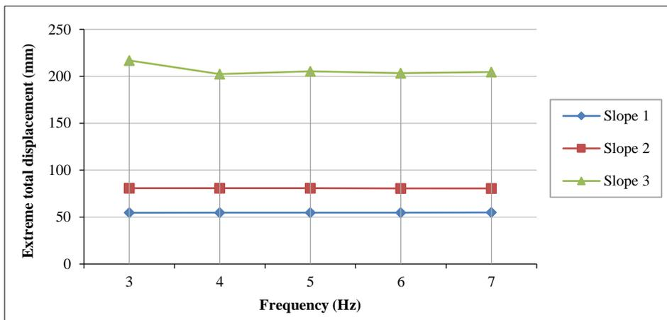
Figure 21. Variation of the extreme total displacement according to an amplitude of 2 mm for the three cases of slope
