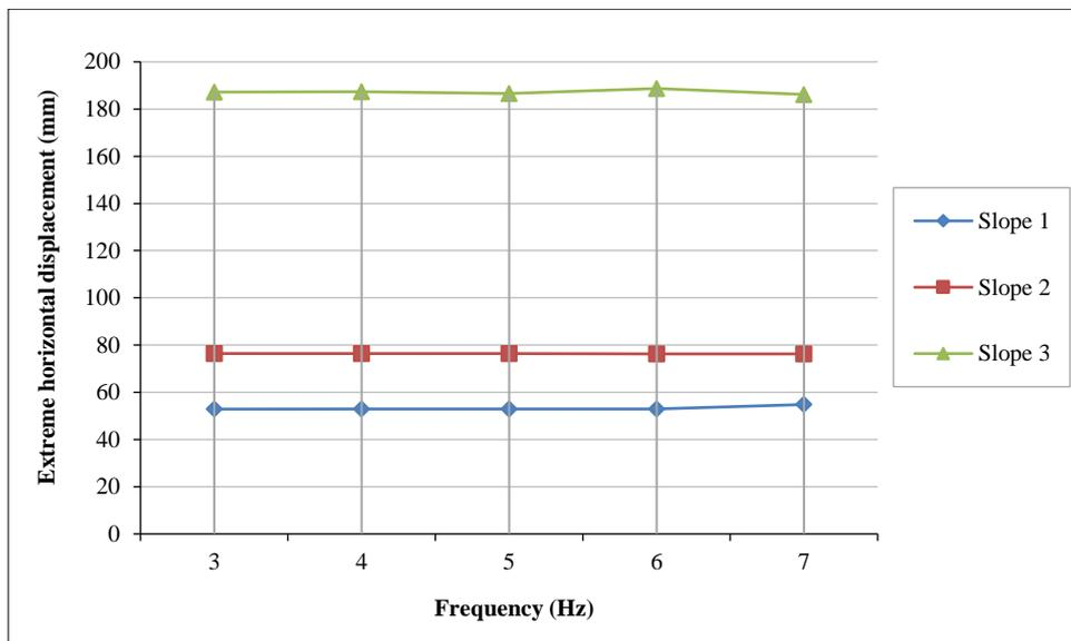
Figure 23. Variation of the extreme horizontal displacement according to an amplitude of 1 mm for the three cases of slope
