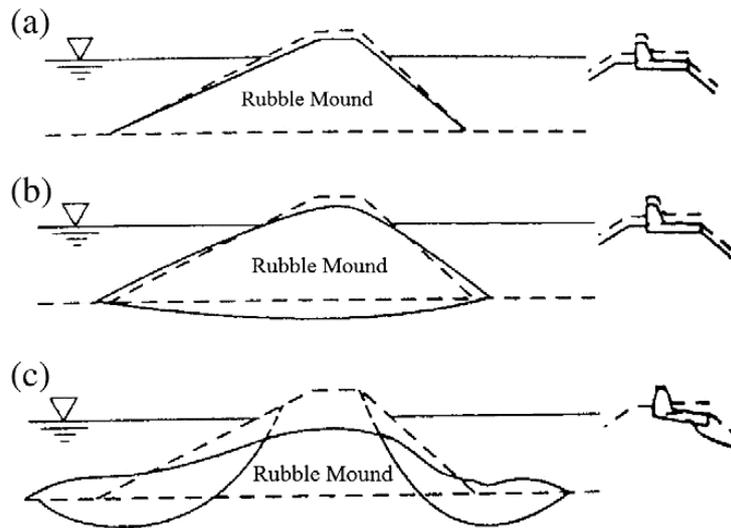
Figure 1. Typical failure modes for rubble-mound breakwaters [18]
