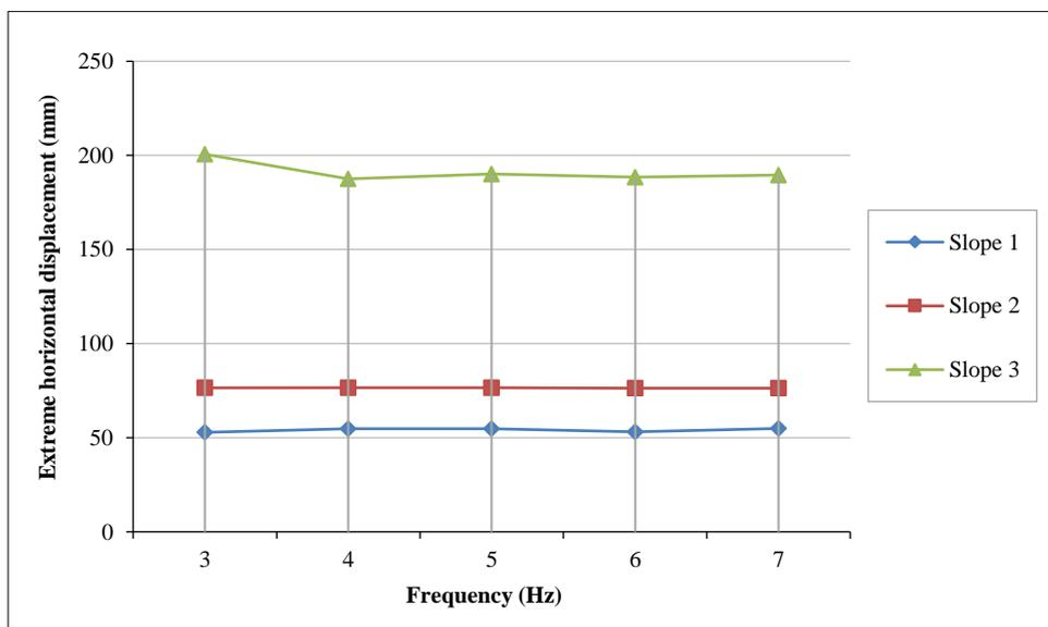
Figure 24. Variation of the extreme horizontal displacement according to an amplitude of 2 mm for the three cases of slope
