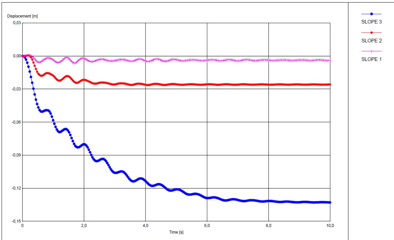
Figure 19. Vertical displacement time history calculated for the three models of breakwater
