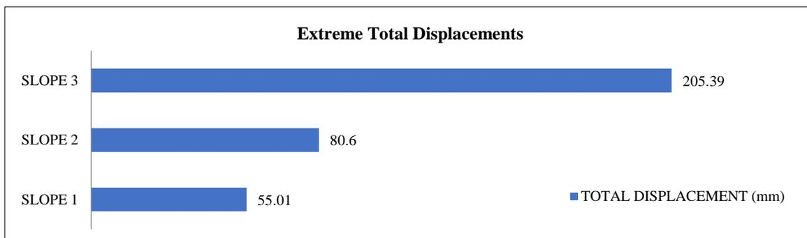
Figure 29. Extreme total displacements of rubble-mound breakwater
