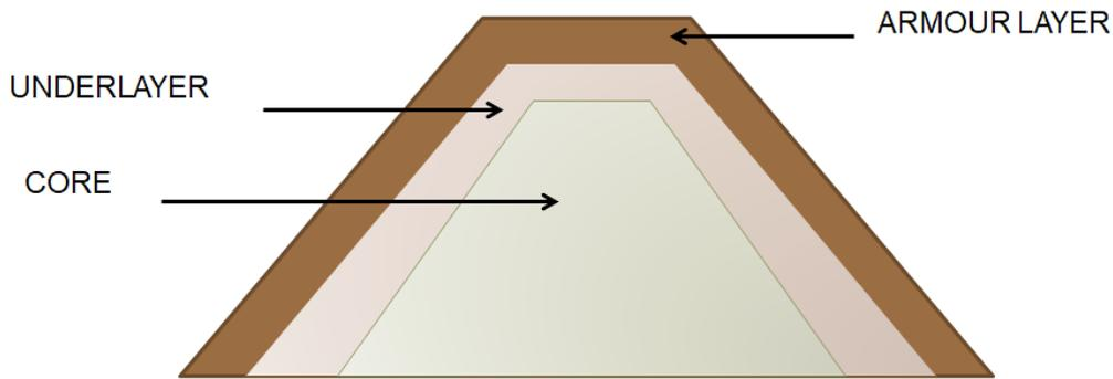
Figure 5. Layer structure of a conventional rubble mound breakwater
