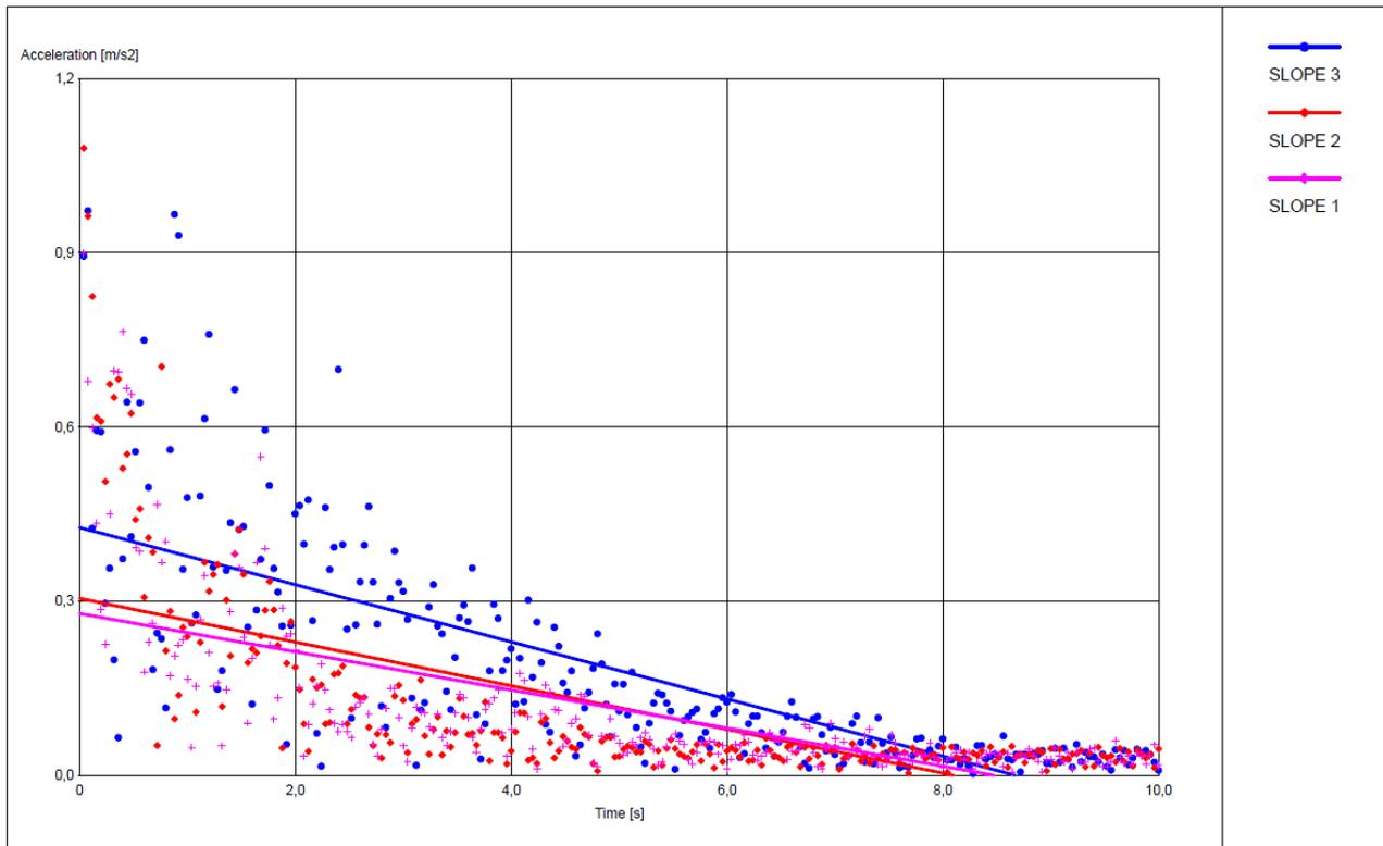
Figure 16. Acceleration time history calculated for the three models of breakwater
