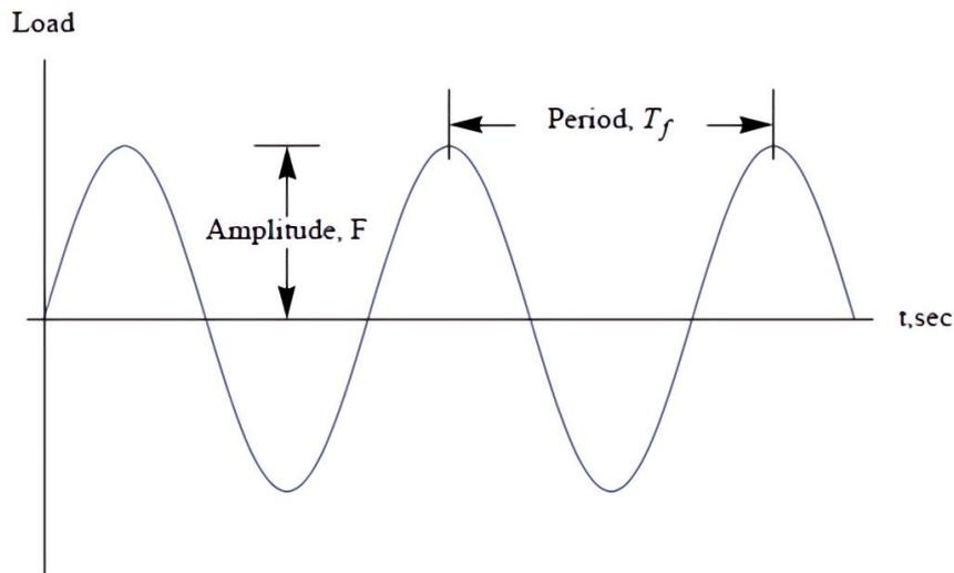
Figure 9. Sinusoidal loading
