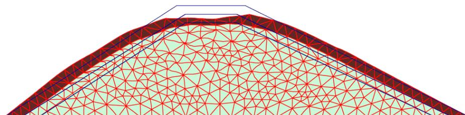
Figure 10. Deformed mesh corresponding to the slope 1
