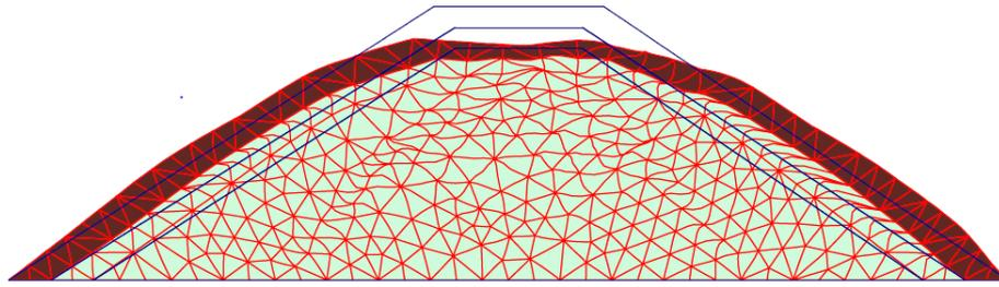
Figure 11. Deformed mesh corresponding to the slope 2
