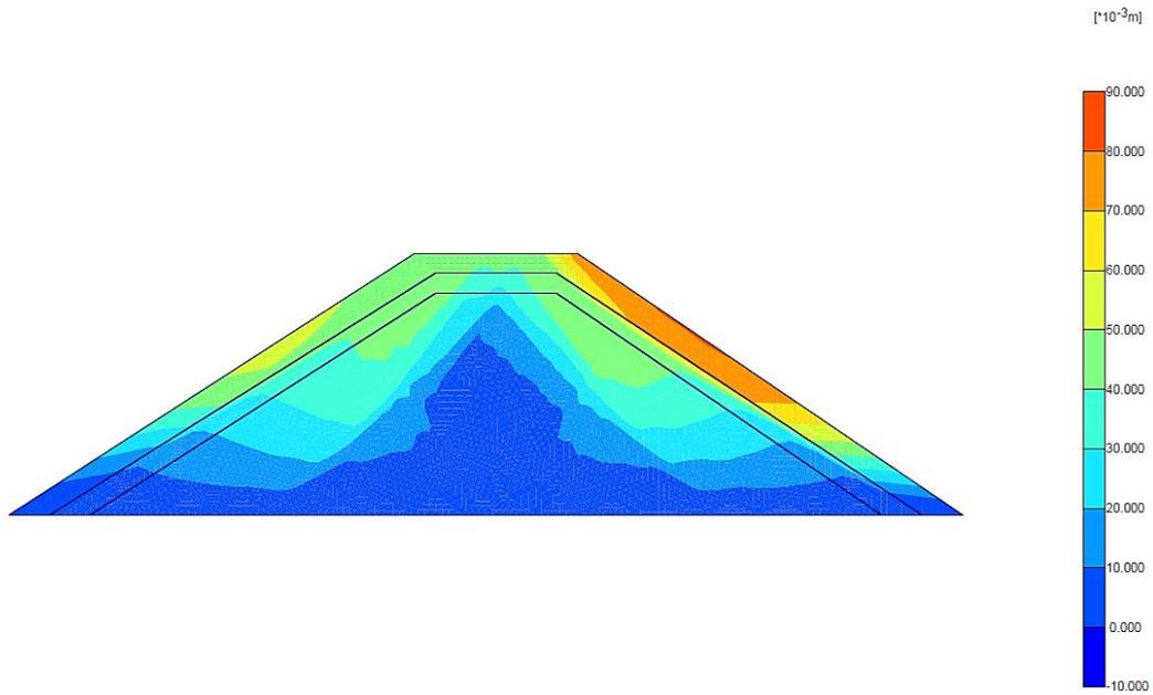
**Figure 14. Contours of extreme total displacement corresponding to the slope 2 after 10s**
