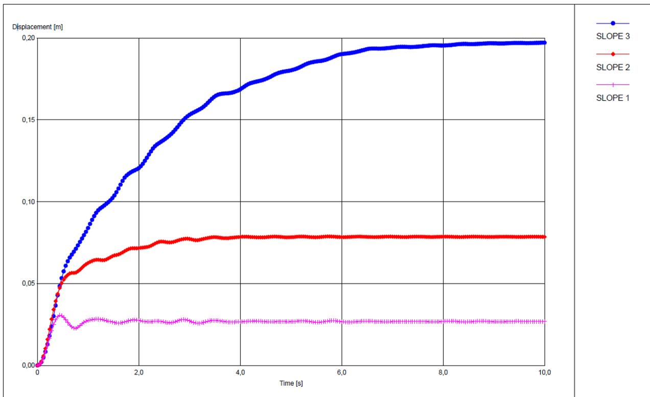
Figure 17. Total displacement time history calculated for the three models of breakwater
