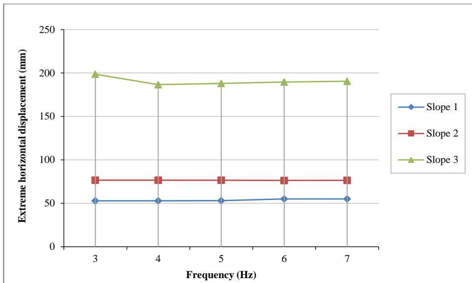
Figure 25. Variation of the extreme horizontal displacement according to an amplitude of 3 mm for the three cases of slope
