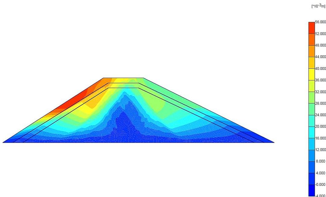
Figure 13. Contours of extreme total displacement corresponding to the slope 1 after 10s
