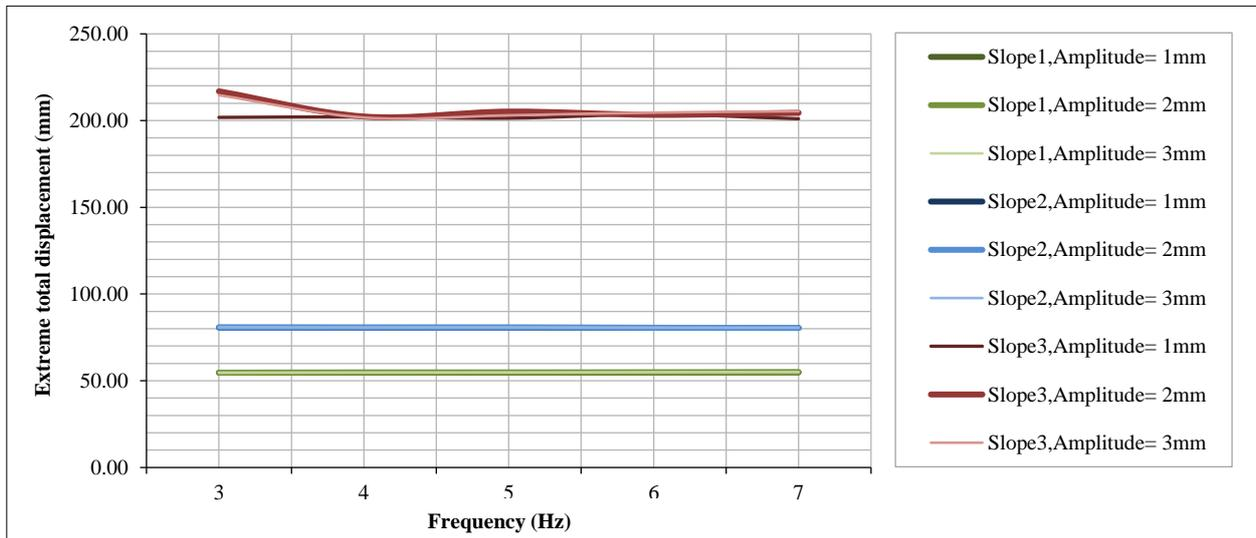
Figure 32. Extreme total displacements corresponding to the three cases for different amplitudes and frequencies
