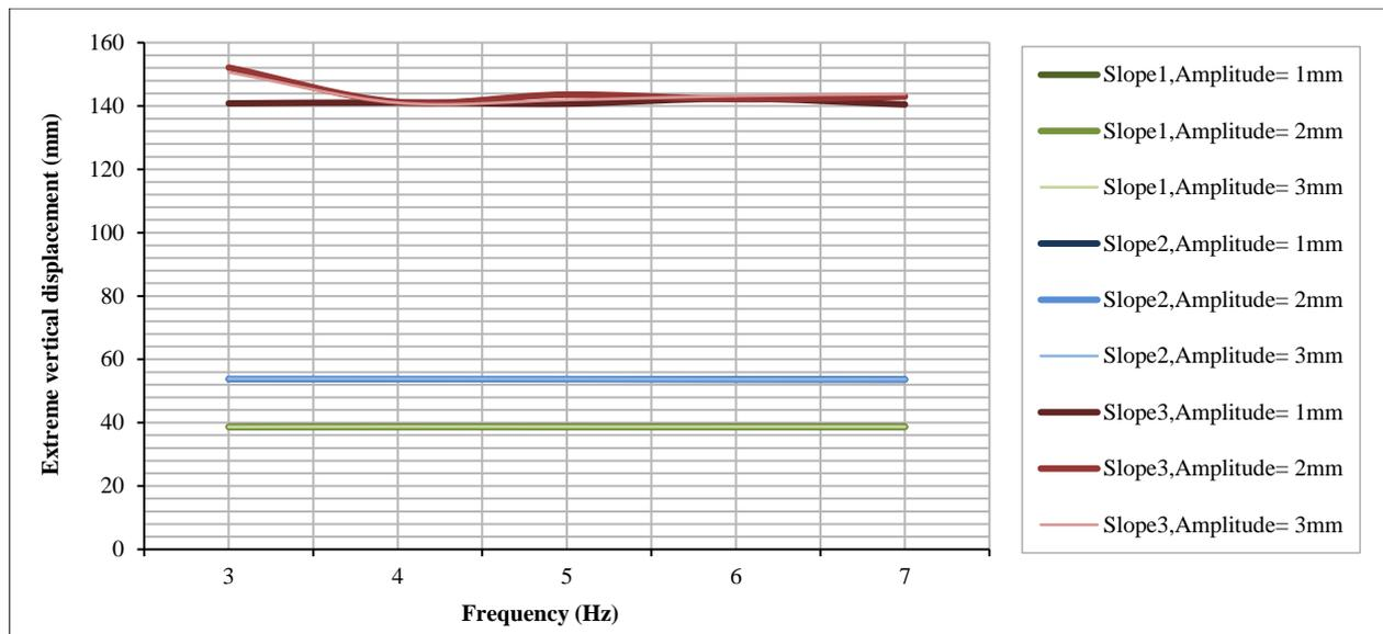
Figure 34. Extreme vertical displacements corresponding to the three cases for different amplitudes and frequencies
