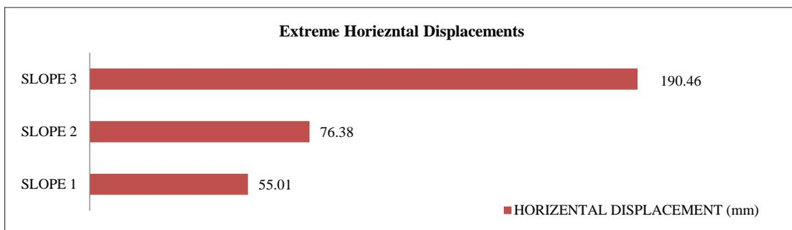
Figure 30. Extreme horizontal displacements of rubble-mound breakwater on seismic's loads
