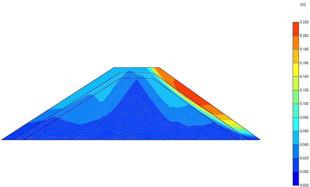
**Figure 15. Contours of extreme total displacement corresponding to the slope 3 after 10s**
