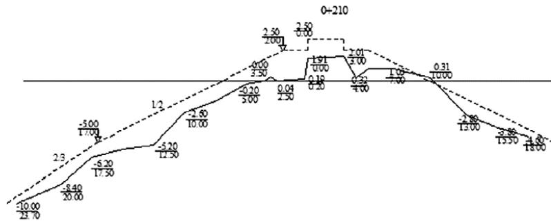
**Figure 3. The settlement of breakwaters after the Kocaeli earthquake, Turkey (1999) [19]**
