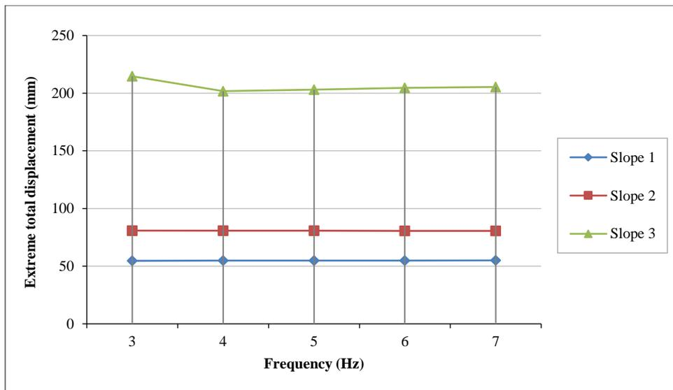
Figure 22. Variation of the extreme total displacement according to an amplitude of 3 mm for the three cases of slope
