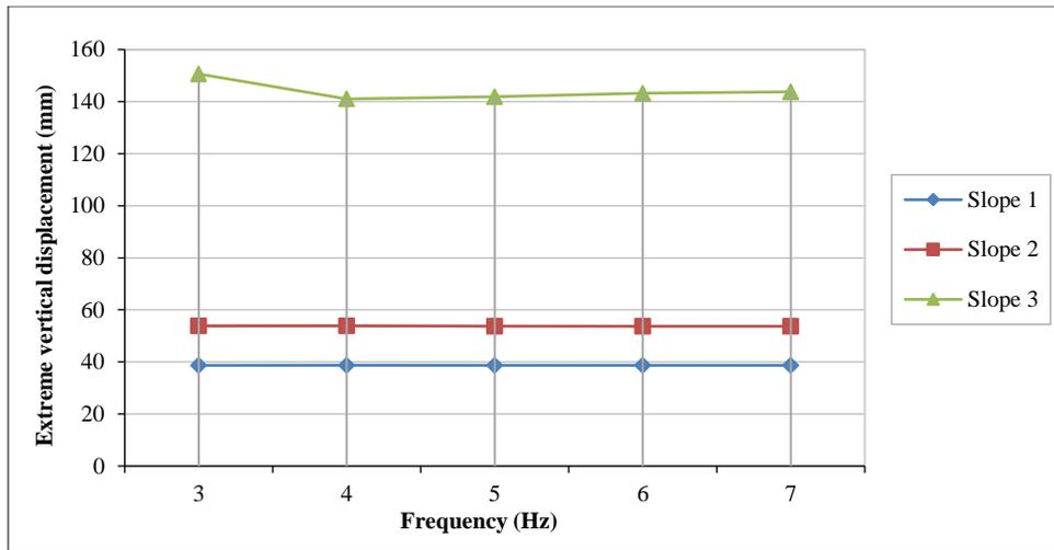
Figure 28. Variation of the extreme vertical displacement according to an amplitude of 3 mm for the three cases of slope
