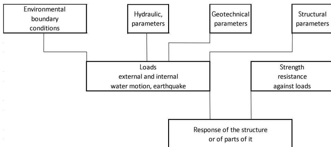
Figure 4. Basic scheme of assessment of rubble mound structure response [29]
