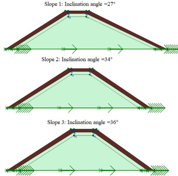
Figure 7. Breakwater model on Plaxis 2D
