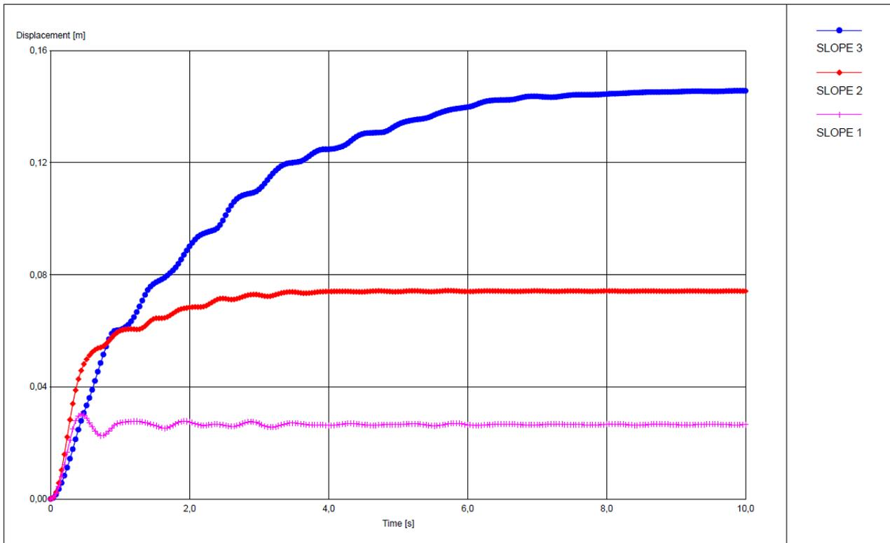
Figure 18. Horizontal displacement time history calculated for the three models of breakwater
