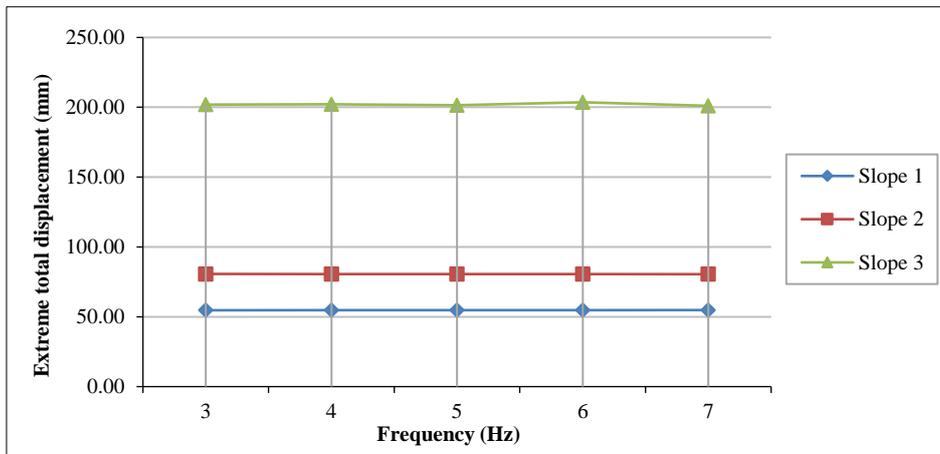
Figure 20. Variation of the extreme total displacement according to an amplitude of 1 mm for the three cases of slope
