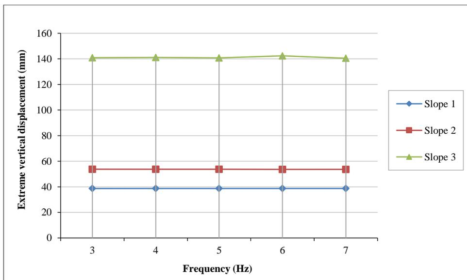
Figure 26. Variation of the extreme vertical displacement according to an amplitude of 1 mm for the three cases of slope
