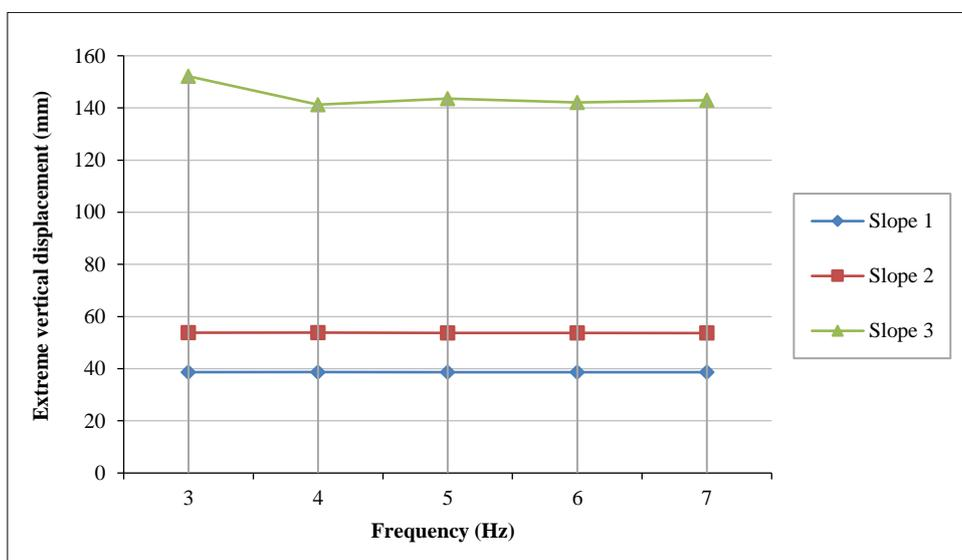
Figure 27. Variation of the extreme vertical displacement according to an amplitude of 2 mm for the three cases of slope
