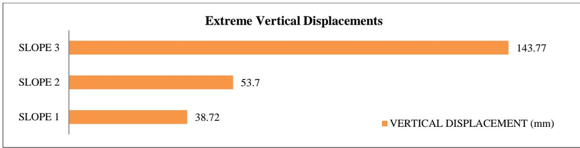
Figure 31. Extreme vertical displacements of rubble-mound breakwater on seismic's loads
