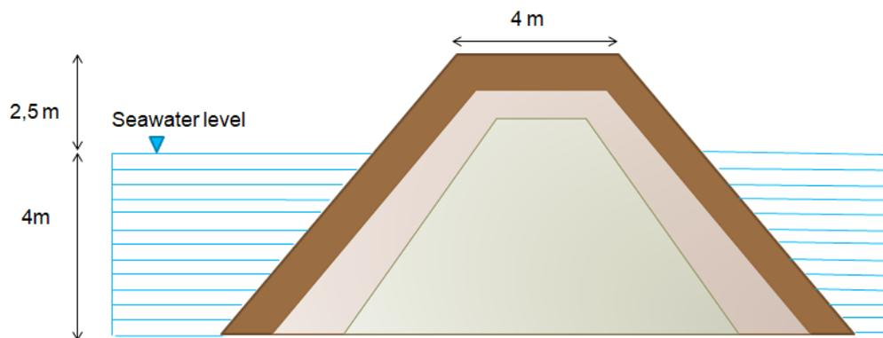
Figure 6. Design of the conventional breakwater
