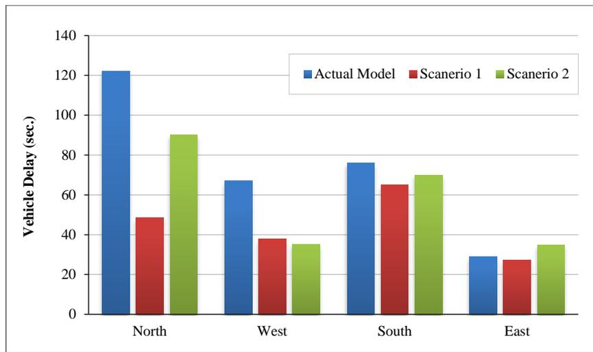
Figure 9. Vehicle Delay Results for Actual Model and Scenario (1) and (2)
