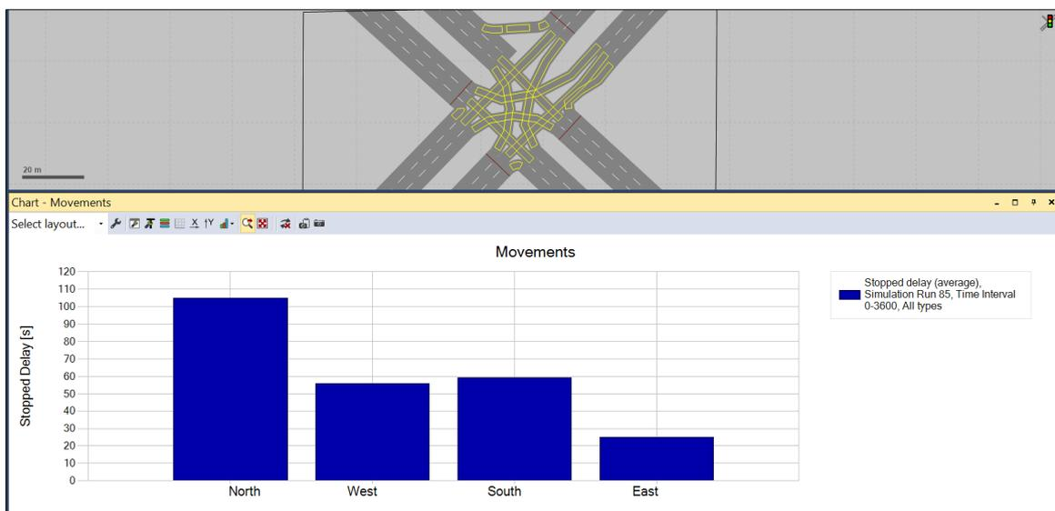
Figure 6. Stopped Delay of Signalized Intersection for All Approaches
