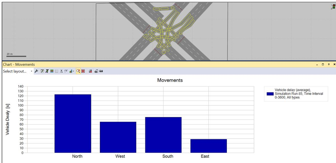
Figure 5. Vehicle Time Delay of Signalized Intersection for All Approaches
