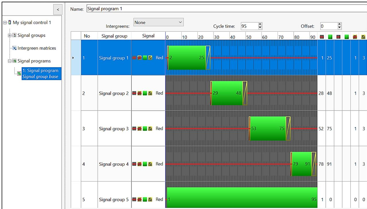
Figure 8. Signal Phase Plan in VISSIM simulation for Scenario (2)
