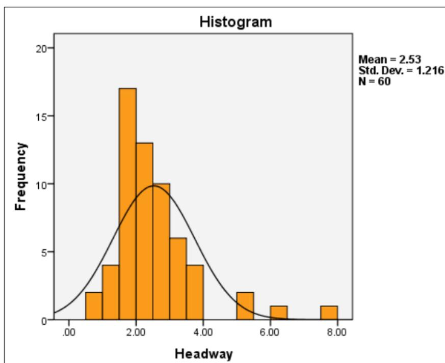
Figure 4. Time Headway Distribution for Signalised Intersection [19]
