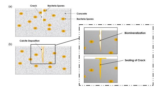
Figure 5. Schematic Illustration of Self-Healing Mechanism: a) crack formation in concrete, b) Bacteria-induced biomineralization process sealing of the crack
