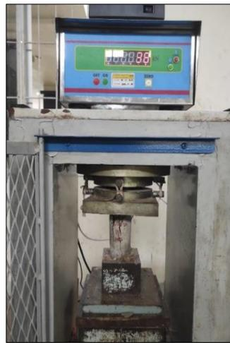
Figure 4. The compressive strength test of mortar
