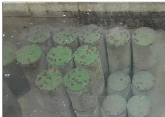
**Figure 2. Water curing in laboratory**
