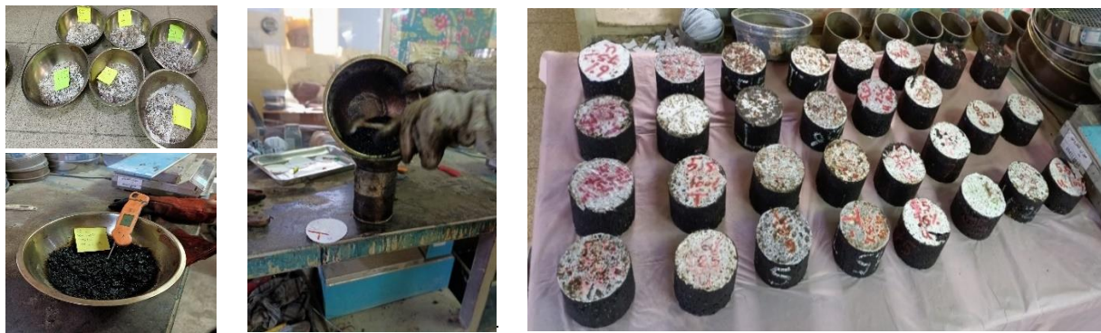
Figure 5. Preparation of Marshall test specimens
