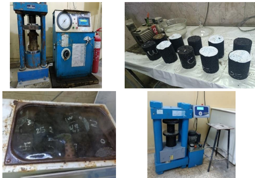
Figure 8. Preparation and testing of compressive strength test specimens
