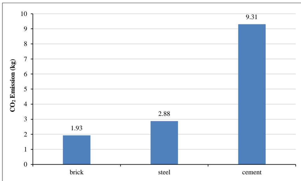
Figure 11. CO<sub>2</sub> emissions by different building construction material
