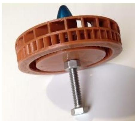
**Figure 25. An impeller for a hybrid mesh turbomachine (prototype version with two rows of blades): a photo of the micromodel – a view from the side of the working medium inlet into the annular channel**
