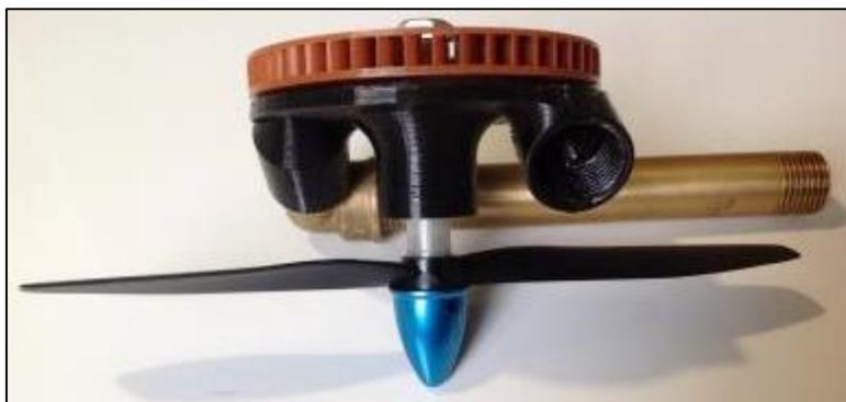
**Figure 9. A photo of a jet system micromodel for energy conversion: a turbofan with a pusher propeller placed at the bottom (prototype version)**
