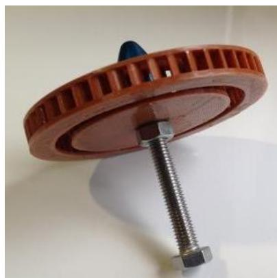
Figure 22. An impeller for a hybrid mesh turbomachine (prototype version according to application 2022110755): a photo of the micromodel – a view from the side of the working medium inlet into the annular channel
