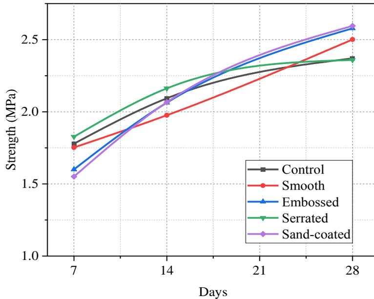
**Figure 11. Split tensile strength results for the different surface modified PET fibres**
