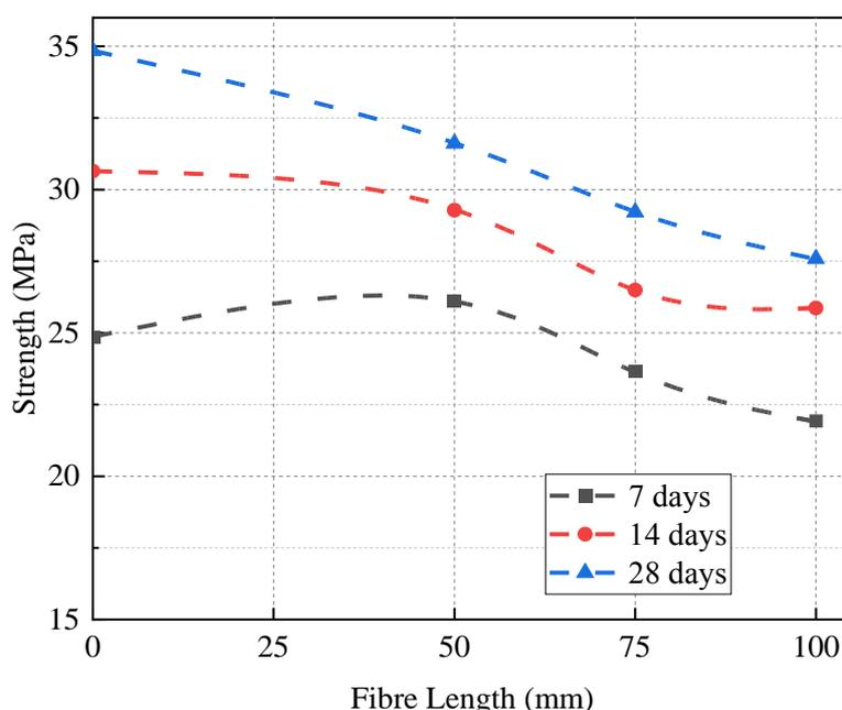
Figure 16. Compressive strength values for varying fibre lengths
