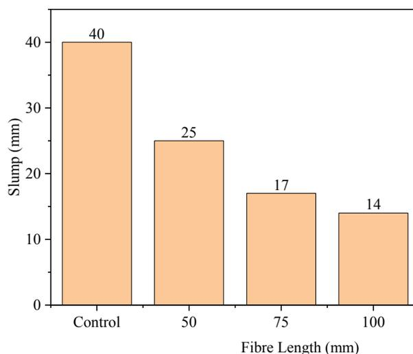
Figure 15. Slump values for varying fibre lengths
