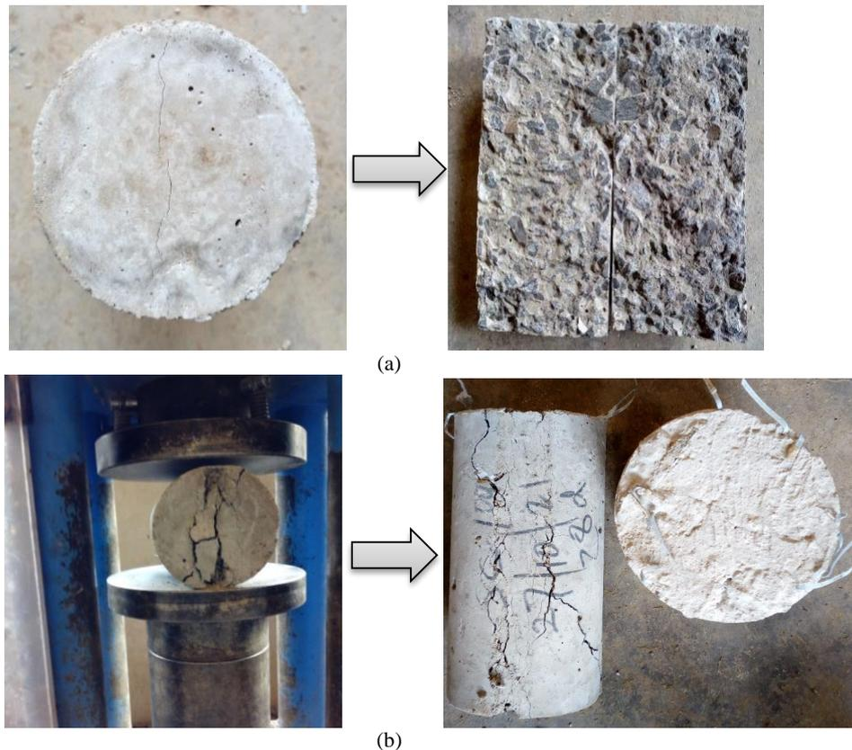
**Figure 12. Failure modes for (a) Control mix without fibres, (b) mix with sand coated fibres**
