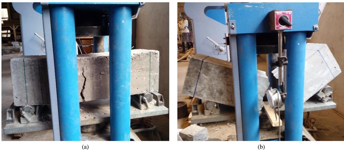
Figure 14. (a) Failure of a fibre concrete specimen (b) Failure of Control specimen (without fibres)
