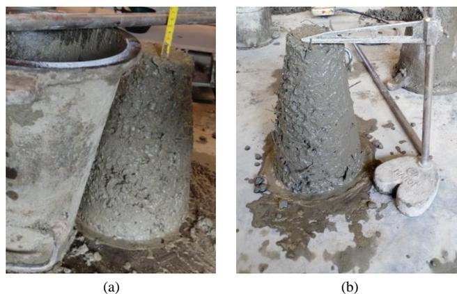
Figure 9. Slump for (a) Control mix; (b) Mix with sand coated fibres
