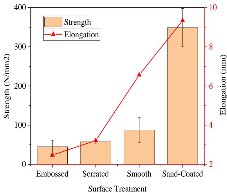
**Figure 7. Tensile strength and elongation for PET Fibres**
