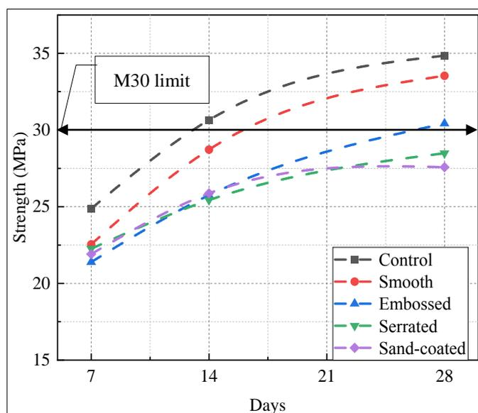
Figure 10. Compressive strength results for the different surface modified PET fibres
