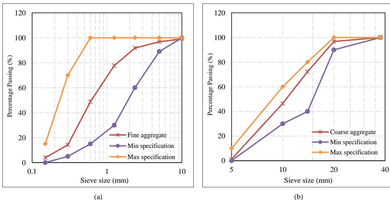
Figure 6. Grading curves (a) Fine aggregates, (b) Coarse aggregates
