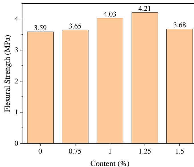
Figure 22. Flexural strength results for varying fibre content
