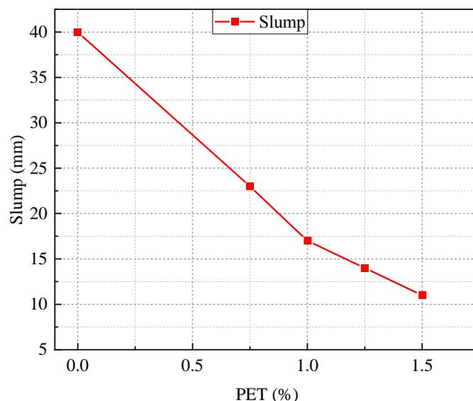
**Figure 19. Slump values for varying fibre content**
