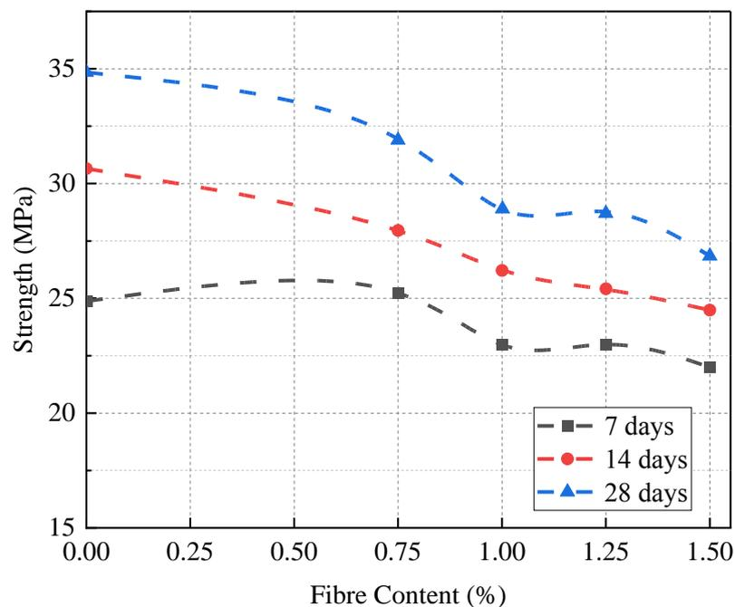
Figure 20. Compressive strength values for varying fibre content
