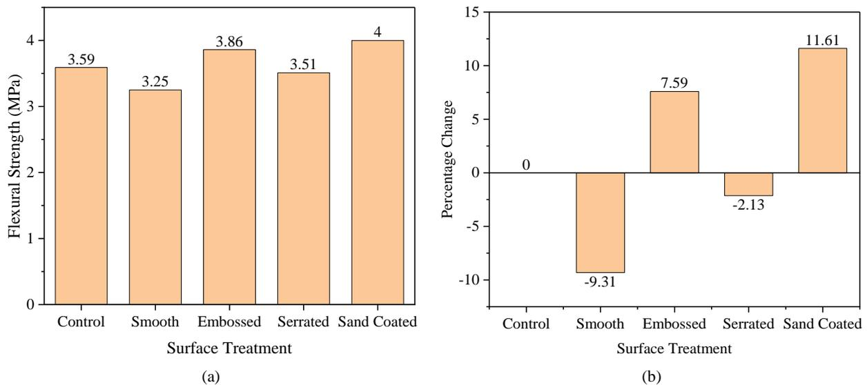
Figure 13. (a) Flexural strength results for different surface-modified fibres (b) Percentage change
