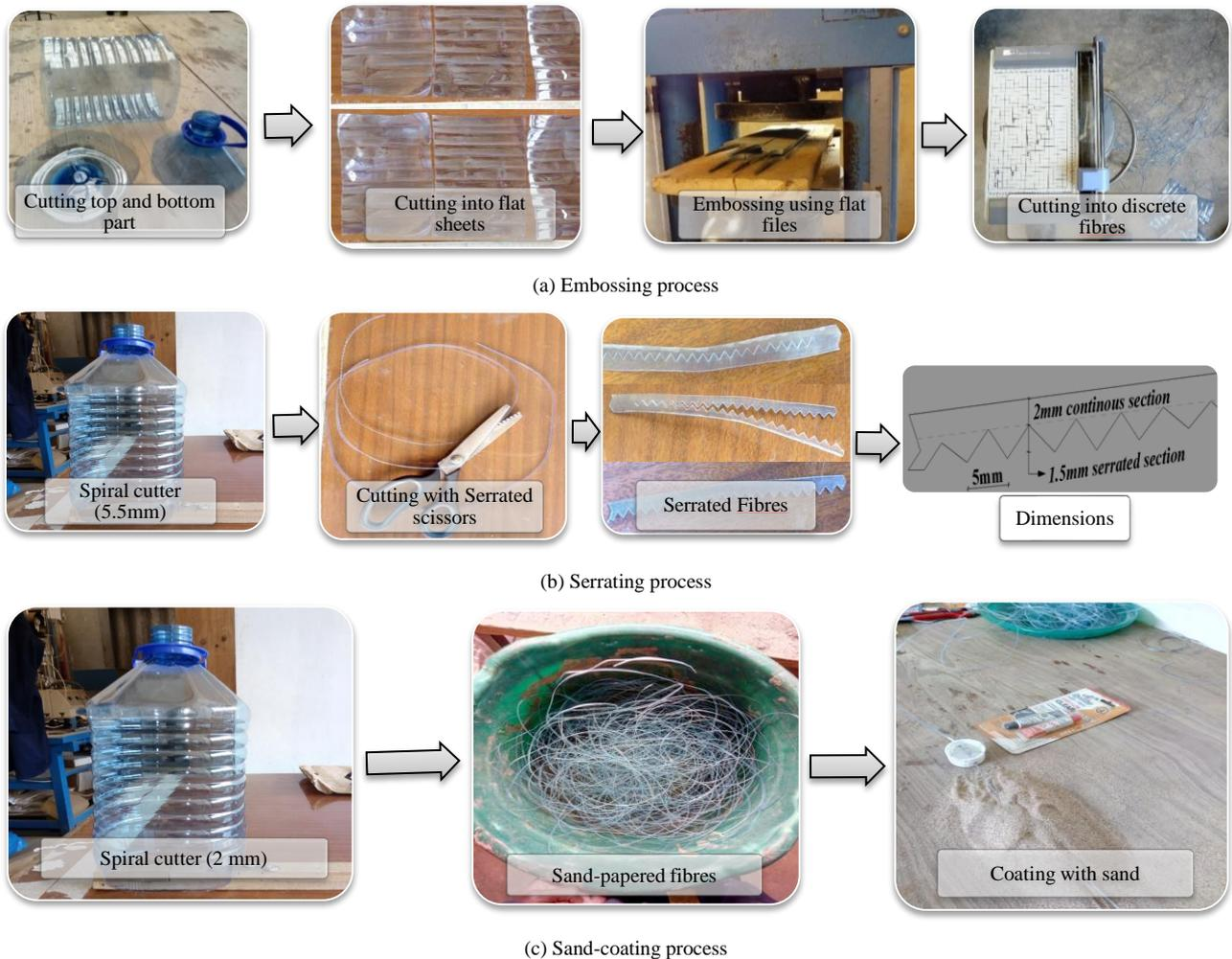
**Figure 3. Preparation of fibres: (a) Embossing, (b) Serrating, (c) Sand-coating**
