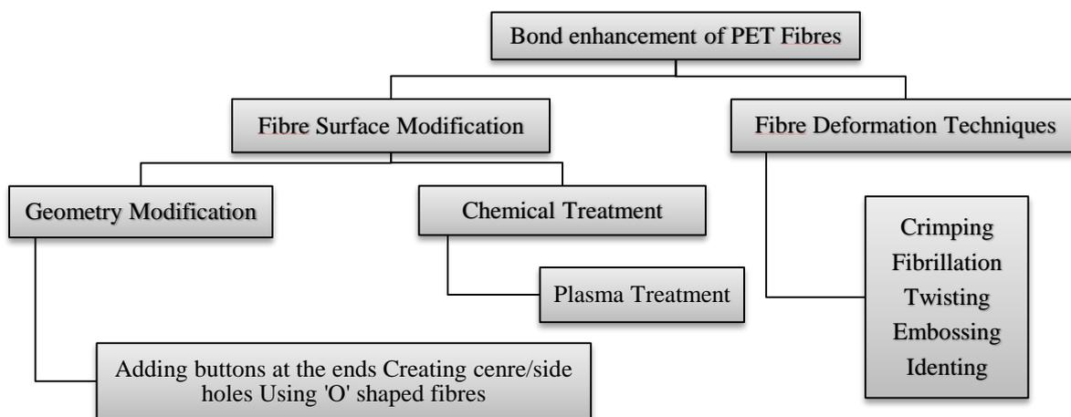
Figure 1. Bond enhancement techniques for PET fibres
