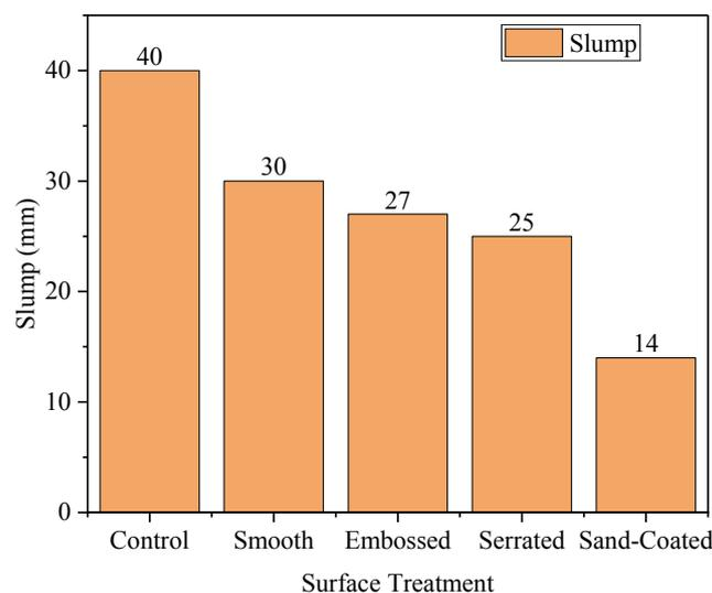
**Figure 8. Slump test results for different surface-modified fibres**
