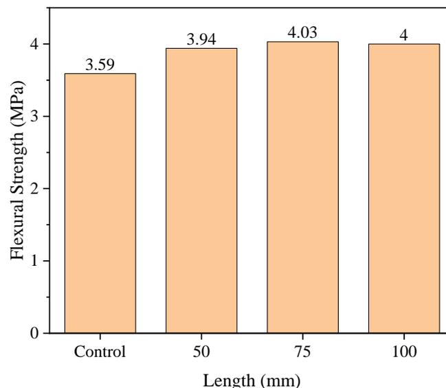
Figure 18. Flexural strength results for varying fibre length
