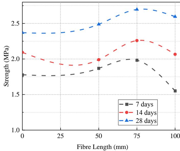
Figure 17. Split tensile strength results for varying fibre lengths
