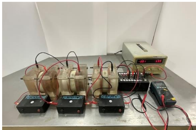
Figure 7. Rapid chloride permeability test apparatus
