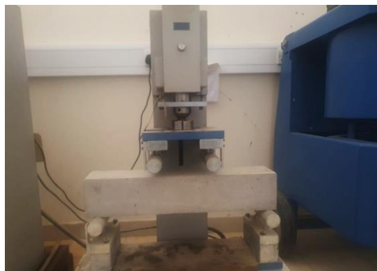
Figure 5. Four point's flexural test
