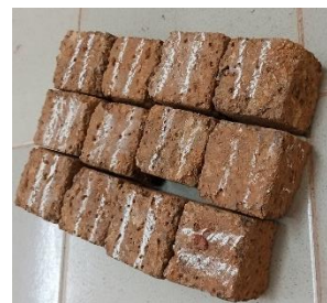
(a) Samples 40 × 40 × 160 (mm) for mortar compression test (b) Samples 70 × 70 × 70 (mm) for compression test on the block
