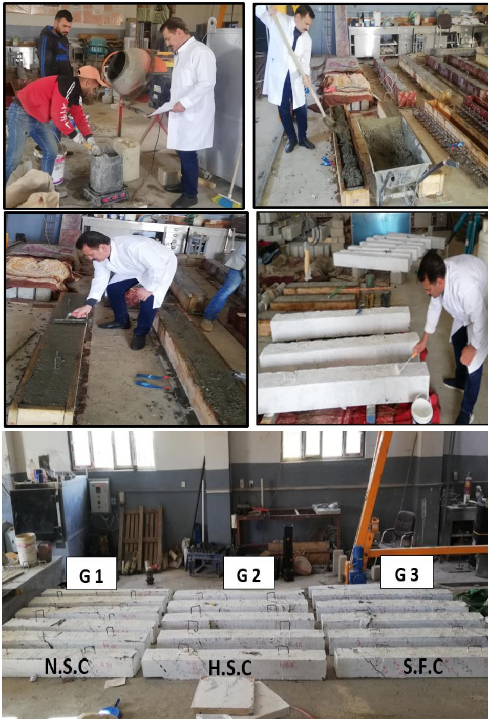
Figure 6. Casting and curing processes of concrete beams
