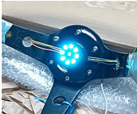
Figure 2. LED ring placement on the steering wheel
