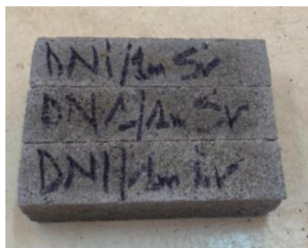
(a) Samples 40 × 40 × 160 (mm) for mortar compression test (b) Samples 70 × 70 × 70 (mm) for compression test on the block
