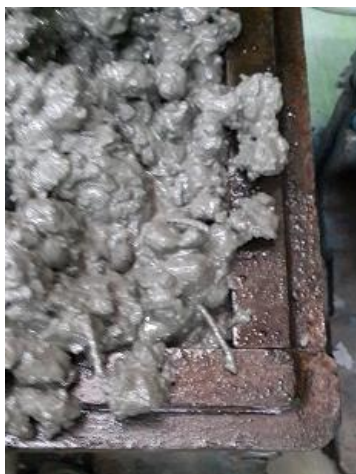
Figure 4. Casting concrete in mould
