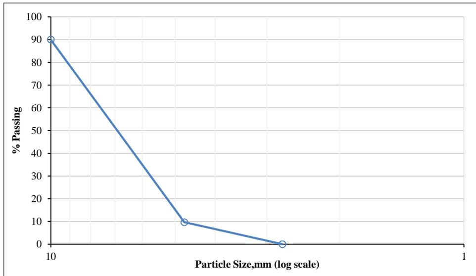
Figure 3. Graph of Particle Distribution of Coarse Aggregate
