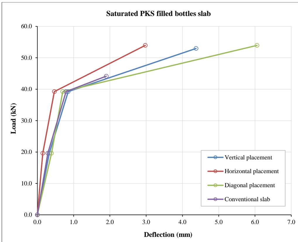
Figure 10. Load Vs. Deflection Behaviour of Conventional Vs. 5% Saturated PKS Filled Bottles Slabs
