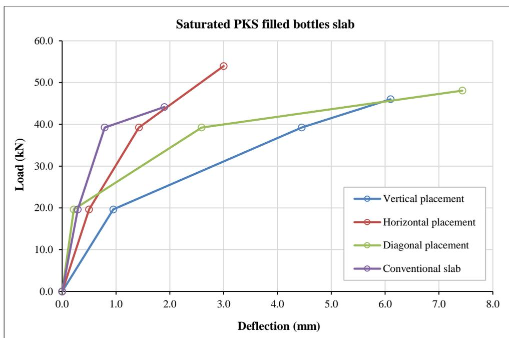
Figure 12. Load vs. deflection behaviour of conventional vs. 10% saturated PKS filled bottles slabs
