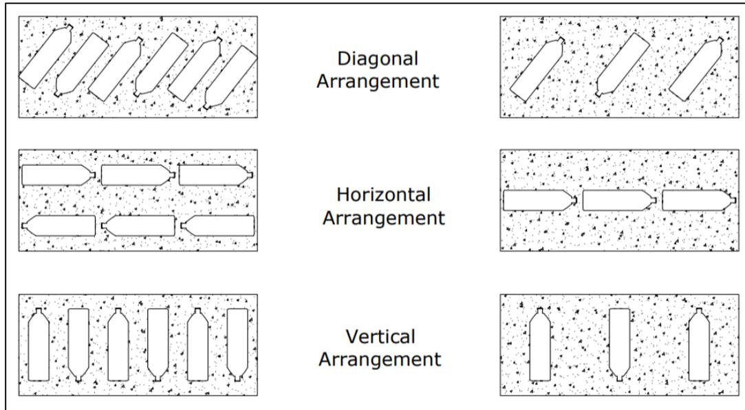
Figure 6. Arrangement of Plastic Bottles in Slab Specimen
