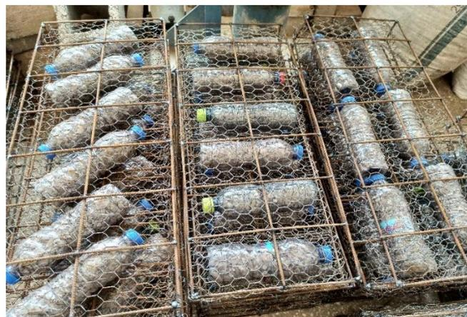
Figure 5. Meshed PKS Plastic Bottles Caged With 8 mm Dia. Steel Reinforcement
