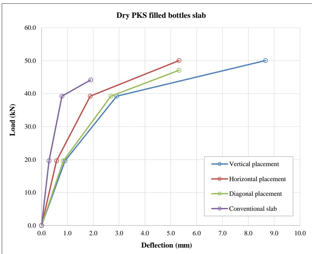
Figure 11. Load Vs. Deflection Behaviour of Conventional Vs. 10% Dry PKS Filled Bottles Slabs
