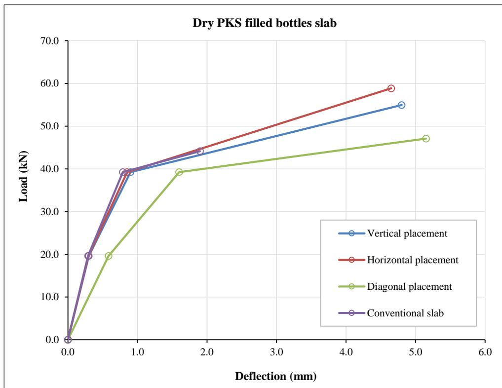
**Figure 9. Load Vs. Deflection Behaviour of Conventional Vs. 5% Dry PKS Filled Bottles Slabs**
