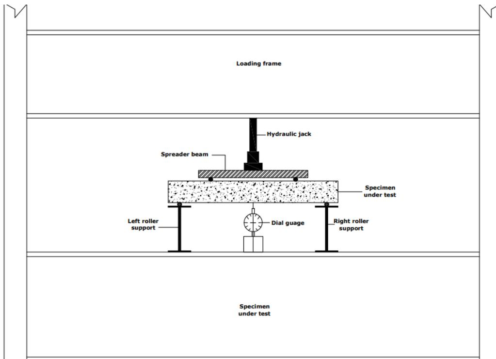
Figure 7. Schematic View of Flexural Strength Test Setup
