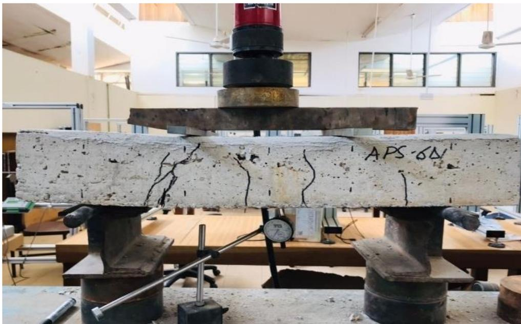
Figure 8. View of Flexural Strength Test in Progress
